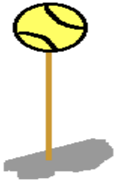
A mass attached to the top of a flexible rod forms an inverted pendulum.
